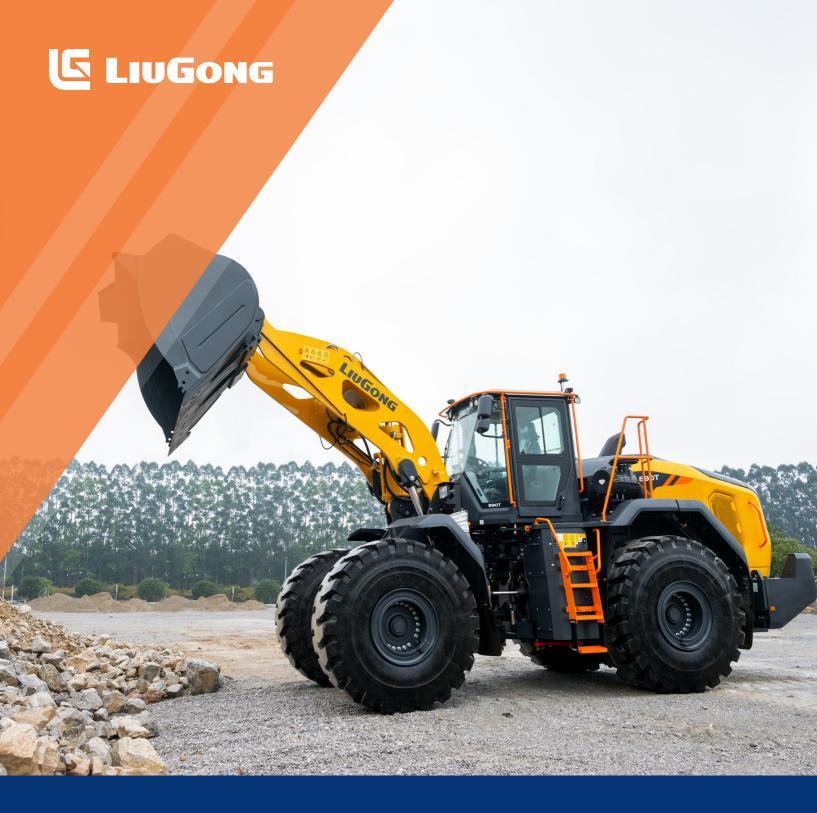
EngineCummins X12Rated Power261 kW (350 hp / 355 ps) @ 2,100 rpmOperating Weight31,750 kg (69,997 lbs)Standard Bucket Size5.4 m³ (7.1 yd³)Standard Breakout Force270 kNStandard Dump Clearance3,332 mm (10'11'')
